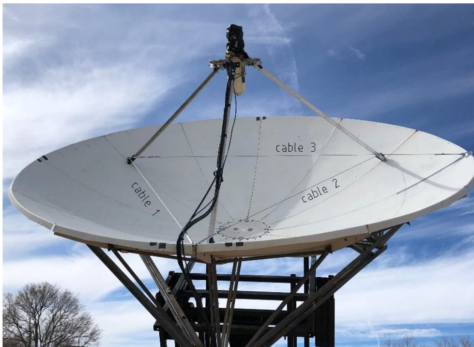
*Fig.10. Image showing locations of the three torsion cables used to adjust curvature of the dish surface.*
