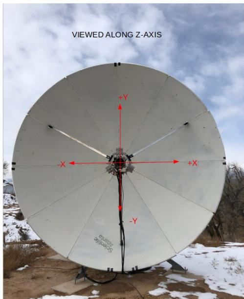
*Fig. 5. Image showing orientation of the x and y axes used during the data analyses.*
