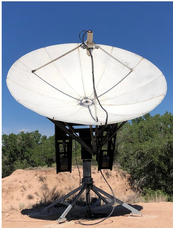
*Fig. 1 The 4.63 meter diameter dish used as the example for this paper.*
